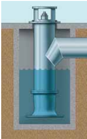
Below Ground Discharge
