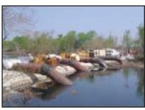
Even before the storm ended, MWI Pump Rental had their Hydraflo™ pumps in route to New Orleans. The Hydraflo™ is a unique, very high volume pump that uses hydraulic power from a drive unit transmitted through flexible hoses to the propeller. This provides great versatility and very quick set up without any type of civil works at all. The Hydraflo™ was invented and patented by David Eller, the CEO of MWI. See the reverse side for more info on why it is such a great pump.
