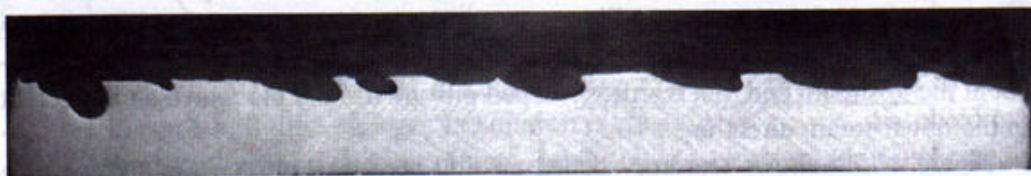
Figure 1: Erosion-corrosion of brass condenser tubing showing individual teardrop shaped pits with undercutting in the downstream direction.
