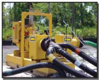
The wellpoint system is used to lower ground water to allow construction of buildings and civil works. All pipes shown bring water from the wellpoints to the suction port in the pump. Discharge from the pump is then either directed to a canal or catch basin depending on site conditions.
